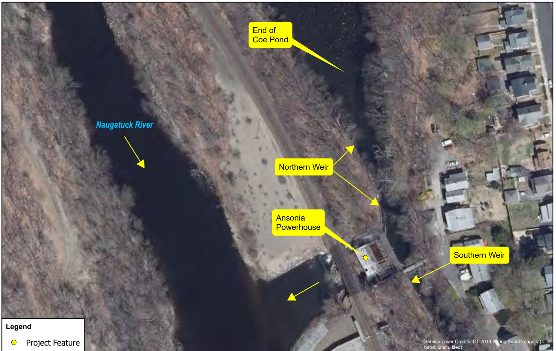
Figure 1.0-3: Project Features at Ansonia Powerhouse
