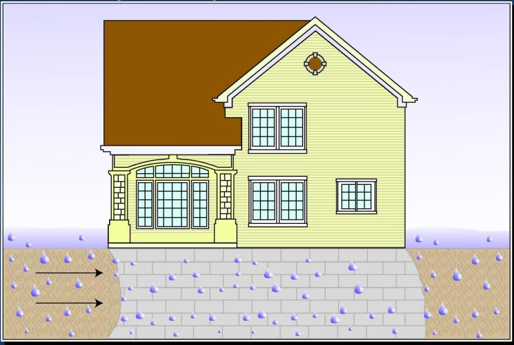
Moving water creates hydrodynamic forces that can create frontal impacts, drag effects, and negative pressure (suction). This can destroy the foundation or move a structure off its foundation.
