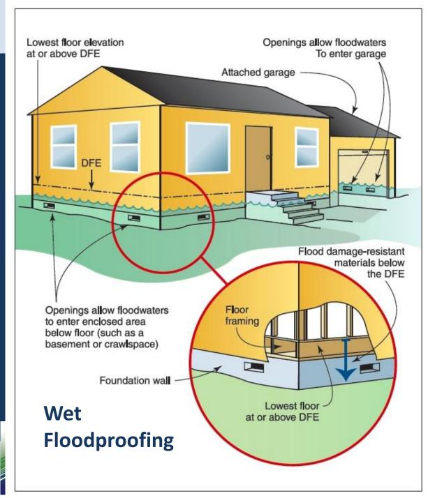
FEMA Technical Bulletin 11-Crawlspace Construction for Buildings in the Special Flood Hazard Area
