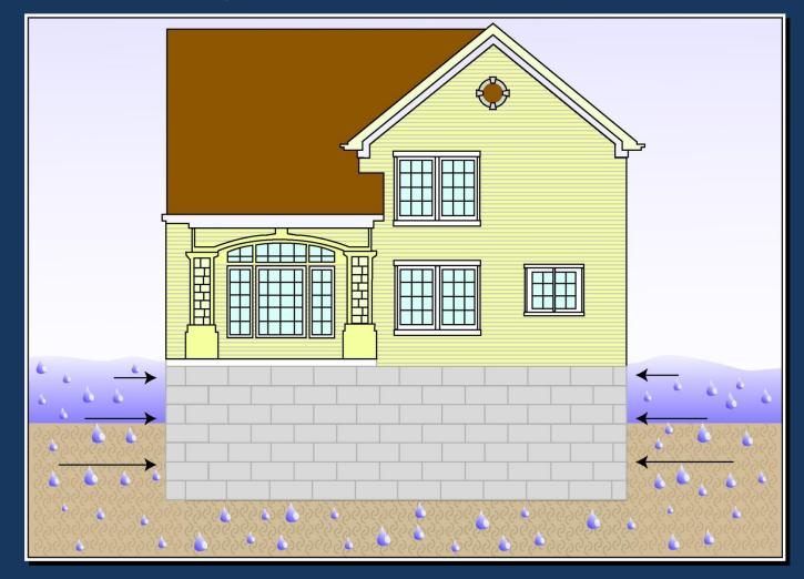
Weight of standing water on a structure exerts a horizontal force. The deeper the water, the more it weighs and the greater the hydrostatic pressure. Installation of flood vents allow pressure to equalize so foundation does not collapse.
