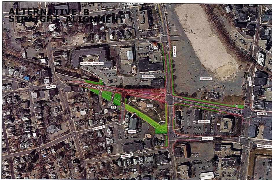
Figure 3 CTDOT Route 72 Realignment Alternative B - Straight Alignment
