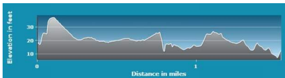
Figure 3-4 Derby to Ansonia Conveyance Pipeline Profile
