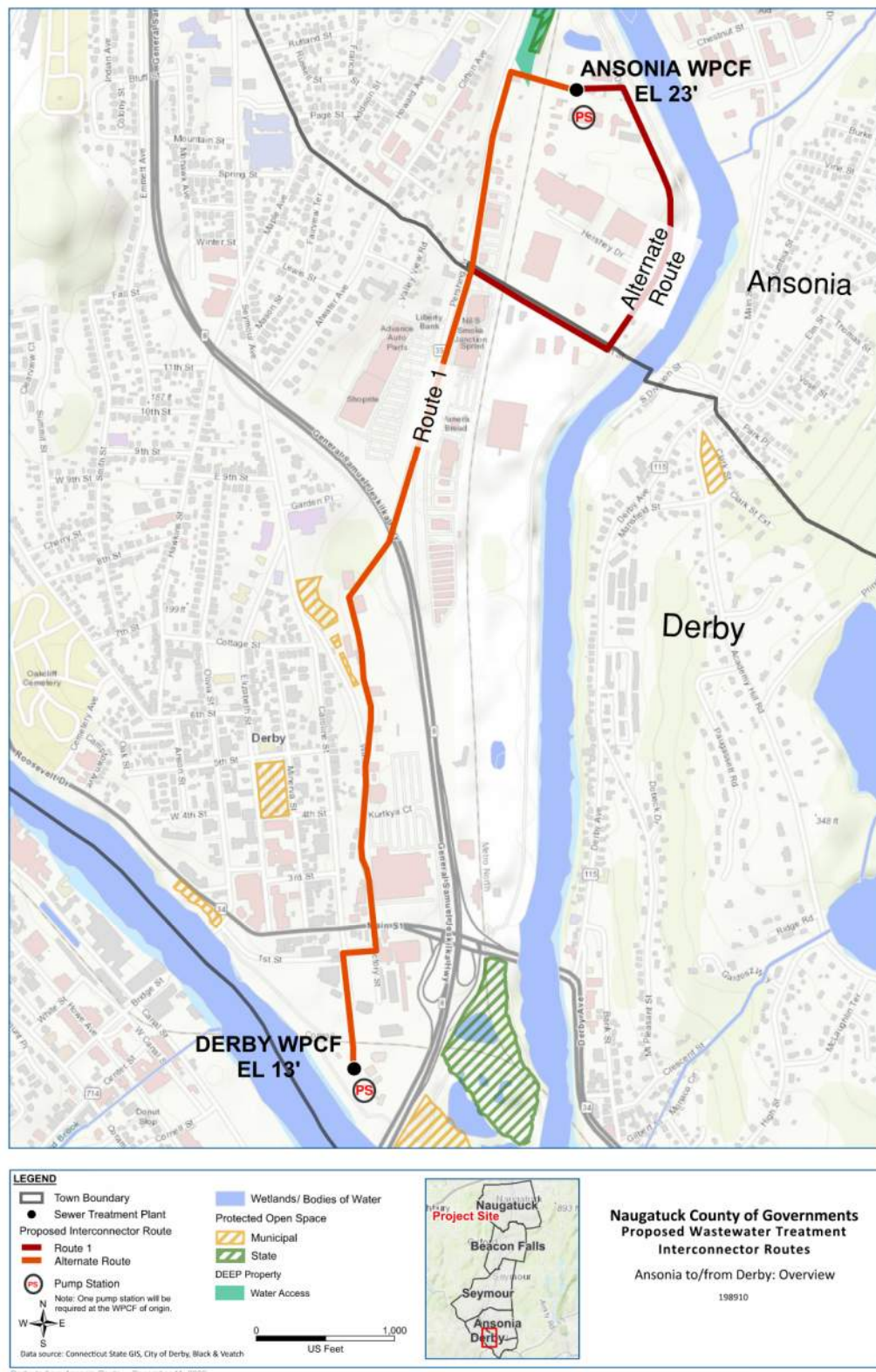
Figure 3-3 Ansonia to/from Derby Conveyance Pipeline Route
