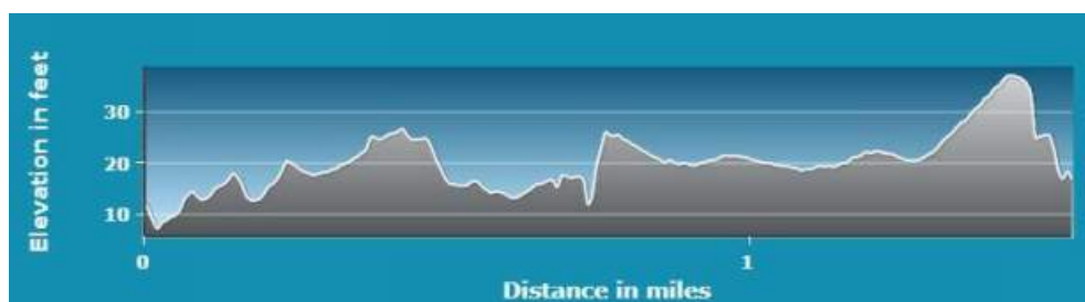
Figure 3-5 Ansonia to Derby Conveyance Pipeline Profile
